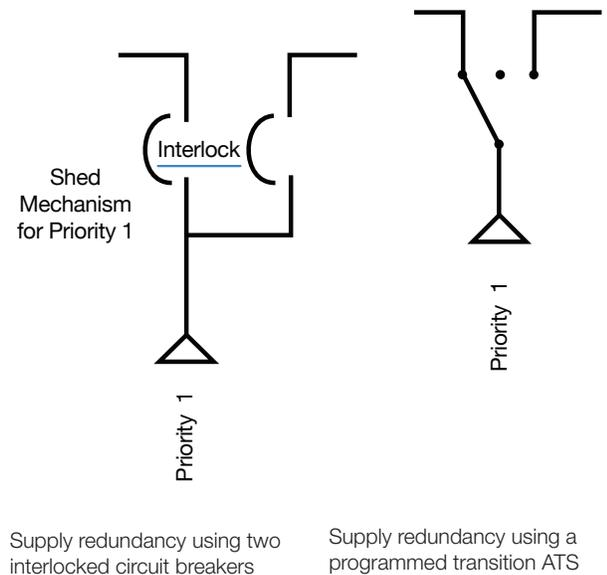
Supply redundancy using two interlocked circuit breakers
